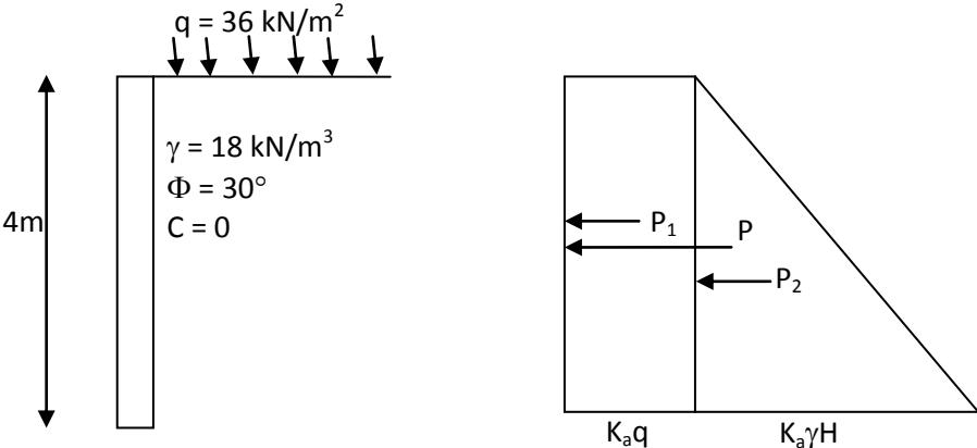
$k_a = \frac{1 - \sin \Phi}{1 + \sin \Phi} = \frac{1 - \sin 30}{1 + \sin 30} = 0.333$ <p>The lateral pressure due to surcharge = <math>k_a \cdot q</math><br/> <math>p_1 = 0.333 \times 36 = 12 \text{ kN/m}^2</math></p> <p>The lateral pressure intensity due to backfill at depth <math>z = 4 \text{ m}</math> is<br/> <math>p_2 = k_a \gamma H = 0.333 \times 18 \times 4 = 24 \text{ kN/m}^2</math></p>                                                                                                 |
