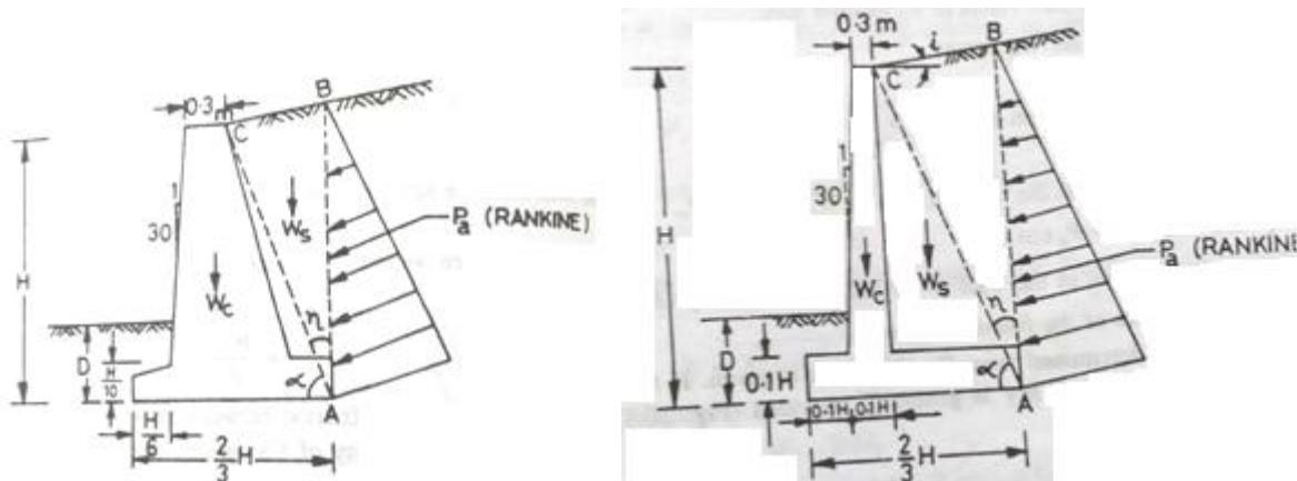
While checking for stability, weight of the soil ( $W_s$ ) above the heel in the zone ABC should also be considered in addition to  $P_a$  on AB and weight of the wall  $W_c$  in case of Rankine's theory.
