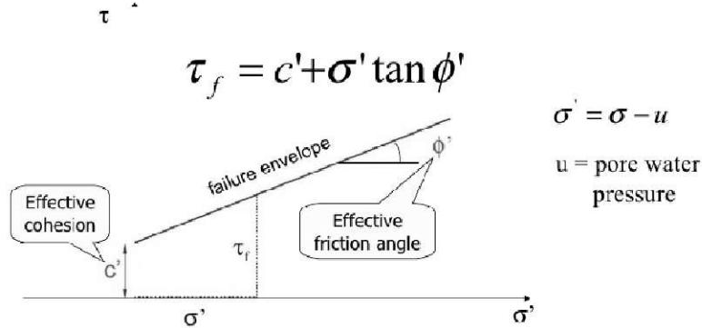
$\tau_f$  is the maximum shear stress the soil can take without failure, under normal effective stress of  $\sigma'$ .
