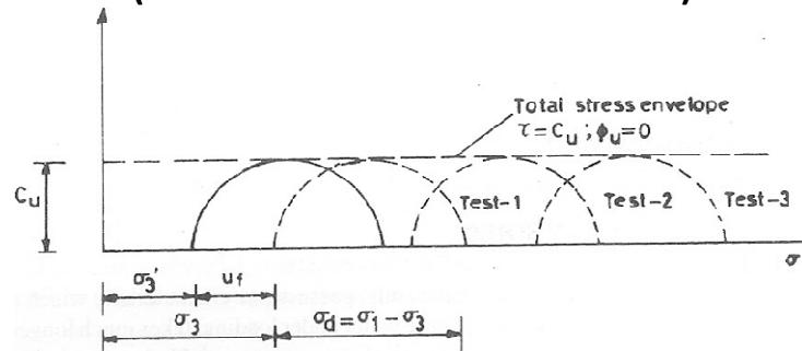
If three tests are conducted on identical samples, each with an increasing confining pressure, **the Mohr circles at failure for all the tests will have the same diameter.**
