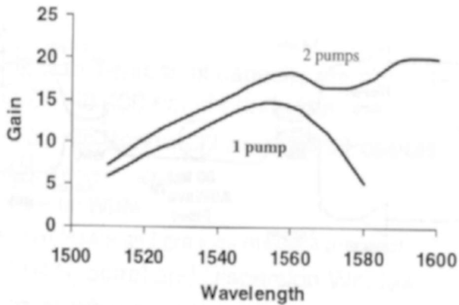
Wide bandwidth Raman amplifier can be realized using multiple pumps
