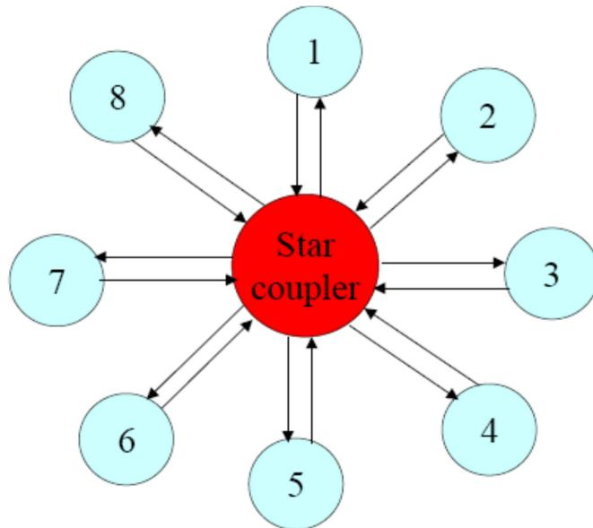
A passive star coupler can be realized with  $N/2 \times \log_2 N$  pcs. Of  $2 \times 2$  couplers
