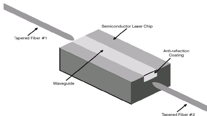
By adjusting the chemical composition of III-V semiconductors (typically Ga In As P) the band gap can be adjusted to give optical gain in the telecommunications windows of interest. The devices are typically 250mm long although devices of up to 1mm have been made. In general the longer devices can achieve higher gain and wider bandwidths.
