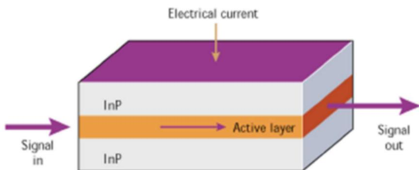
Semiconductor optical amplifiers, like their semiconductor-laser, consist of gain and passive regions. Layers of antireflective coatings prevent light from reflecting back into the circuit while the incoming signal stimulates electrons in the gain region.
