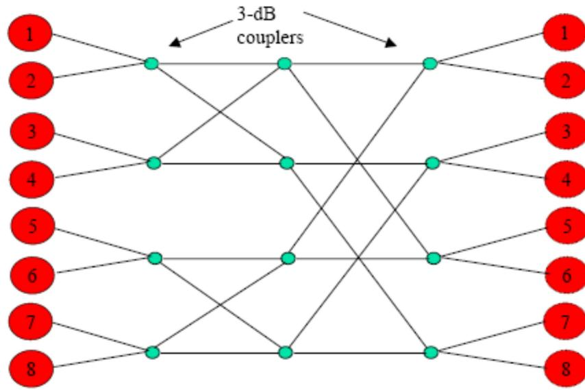
Each signal passes through exactly  $\log_2 N$  couplers, thus the loss is uniform for all nodes (assuming that there is no insertion and other losses, each signal experiences  $3\text{dB} \times \log_2 N$  loss). The coupler is a passive element, so no external power is required to establish such a hub.
