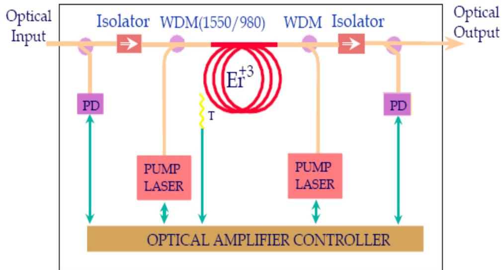
When you actually look at an EDFA block diagram you see the input on the left the output on the right, photo diodes to measure input and output power levels, pump lasers which are used to excite this piece of erbium doped fiber to a higher energy state, and 1550 light is allowed to pass through.
