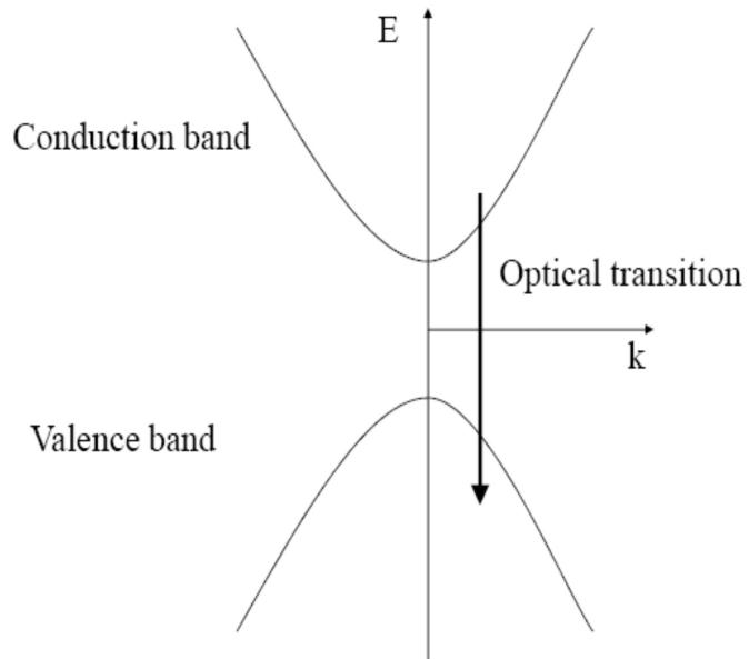
The DC current applied to the device results in electrons being pumped into the (normally empty) conduction band and removed from the (normally full) valence band. This creates the population inversion which is a pre-cursor to optical gain. When signal photons travel through the device they cause stimulated emission to occur when an electron and hole recombine.
