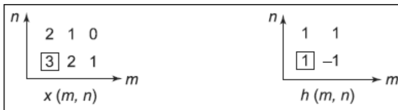
FIGURE 3.8(a) The functions x(m, n) and h(m, n) used for convolution
